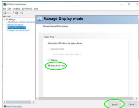
Figure 10 - Manage Display Mode - NVIDIA GPU only
